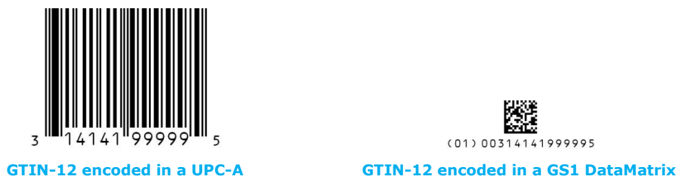
Figure 6-3 GTIN-12 in a UPC-A and GS1 DataMatrix
