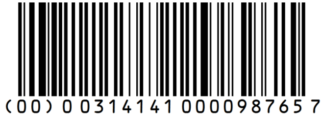
Figure 6-4 SSCC Encoded in a GS1-128
