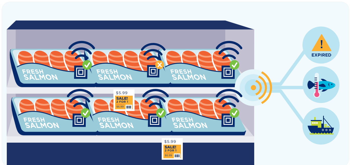
Figure 3: Detecting the presence of expired perishable foods using shelf-embedded RFID tag-based gas sensors
