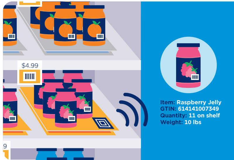
Figure 2: RFID enhanced pressure pad for weight detection
