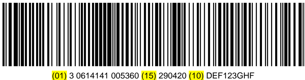
Figure 5. Sample GS1-128 barcode with GTIN (01), Best Before Date (15), and Batch/Lot Number (10)
