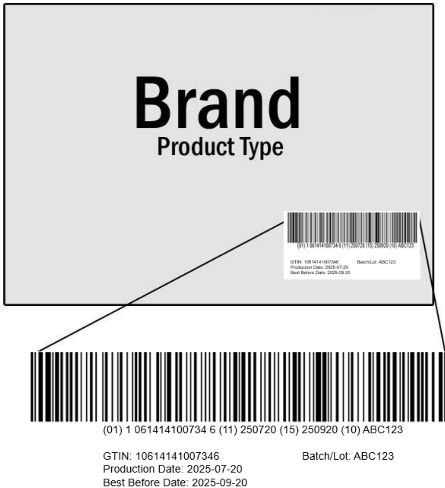
Figure 17. Sample case label showing the use of GS1-128 barcode and human readable text to communicate GTIN (01), Batch/Lot Number (10), Production Date (11), and Best Before Date (15)
