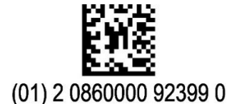
Figure 6d: GTIN-14 in a GS1 DataMatrix Barcode (DI only or PI can be added as shown in 6c)
