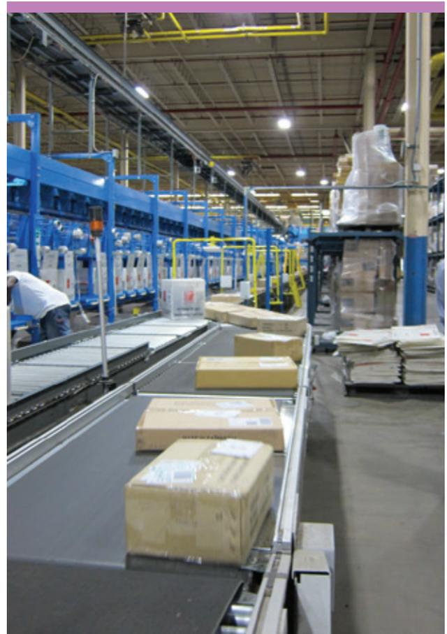
Warehouse and conveyor automation enabled with RFID.
