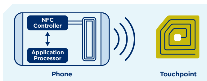
Figure 6: All smartphones are equipped with the ability to read and process NFC tag data.
