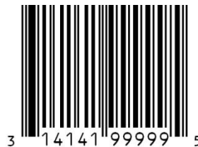
Figure 6-3 Example of a UPC-A Barcode Used for POS and/or U.S. FDA Barcode Rule
