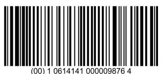
Figure 2-1 GS1-128 barcode containing SSCC
