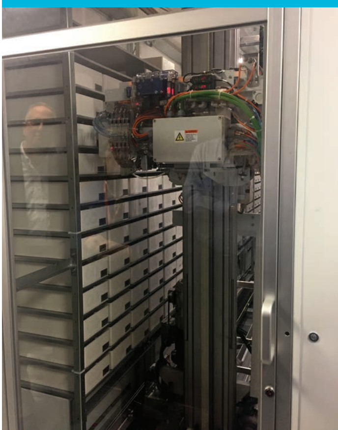
Automated box-picker within commercial drug storage unit at Dana-Farber.
