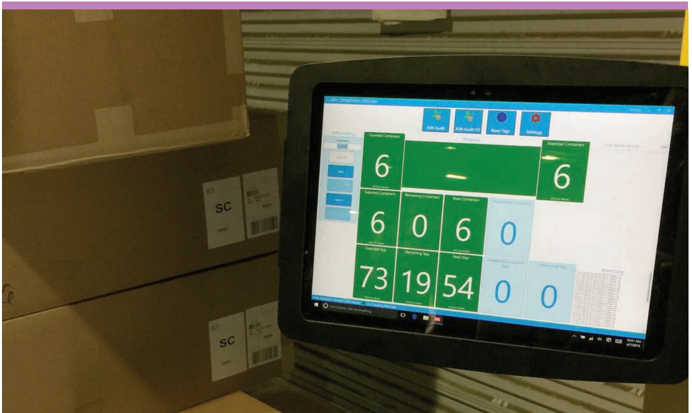
In the shipping area, clerks punch in the ASN number to verify the right cartons with the right products are being loaded on trucks bound for customers.
