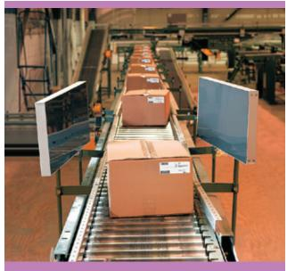
Case-level scanning at a brand owner's distribution center via a conveyor RFID tunnel.
